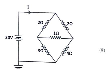
(b) Find out source current  $I_s$  and current through the resistance  $2\Omega$   $(I_{2\Omega})$  in the circuit given below.
