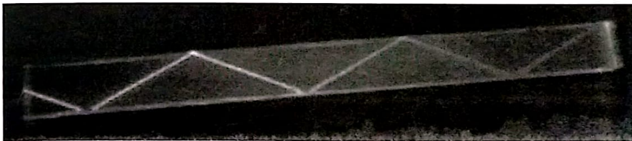
Figure 1. Light propagation through planar optical waveguides
