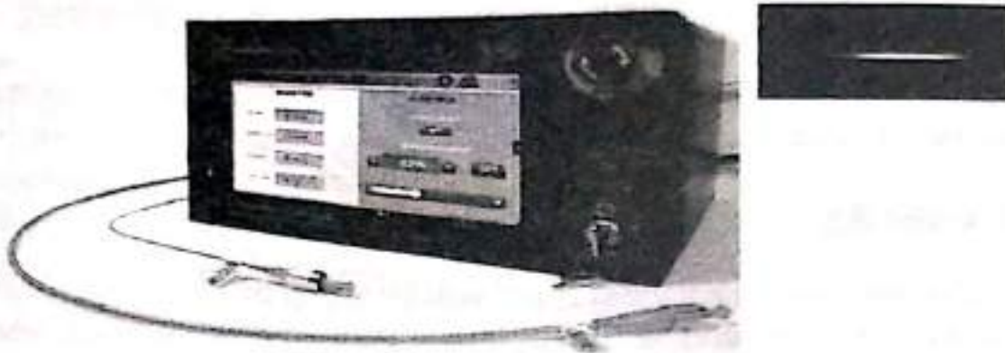
Figure 27: Commercially available supercontinuum white light source produced by VINVISH Technologies, Trivandrum and CGCRI, Kolkata; photograph courtesy: Dr. Shyamal Bhadra and Dr. Ramadas Pillai.
