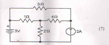
(b) Obtain Norton equivalent circuit for the network external to the  $3\Omega$  resistance for the given network. Further determine the current through  $3\Omega$  resistor.
