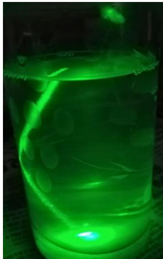
Figure 6. Demonstration of Total Internal Refraction in a glass filled with liquid
